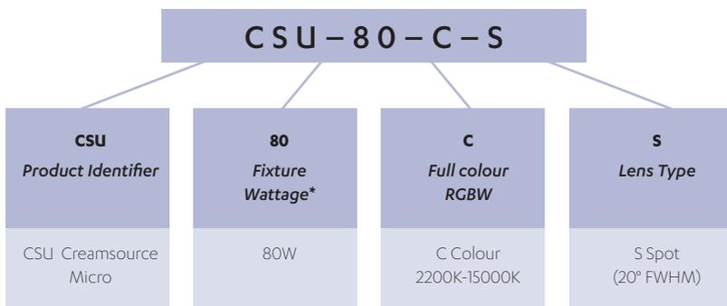
When supplied as a complete kit, including power supply and cables, the part number will have a K as a prefix. Check [www.outsight.com.au](http://www.outsight.com.au) for up to date list of kitting options and part numbers.
