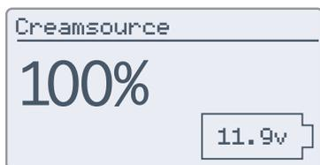
If the input voltages falls within 10% of the user-definable Shutdown Voltage, a flashing battery icon will displayed.
