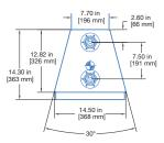
The UPA-1P loudspeaker provides high power output, low distortion, and consistent polar response in a compact, vented two-way enclosure. The loudspeaker features a 12 in cone low-frequency driver and a 3 in diaphragm compression driver coupled with a 100° horizontal by 40° vertical constant-Q horn. The versatile UPA-1P has a variety of sound reinforcement applications including as a main front-of-house loudspeaker in small- to mid-sized venues and as a fill loudspeaker in larger systems.
