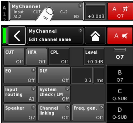
Selecting a particular channel from the Home screen opens the corresponding Channel setup screen with the respective Channel tab being active.
