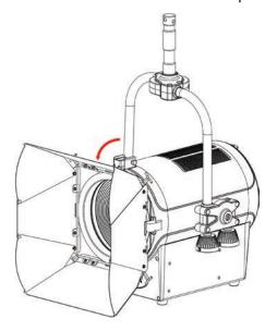
2. Slide the barn door into place in one of the vacant accessory slots on the front of the fixture.
