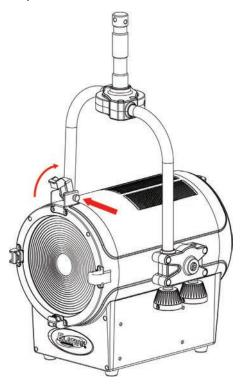
3. Return the retaining clip to the original position to lock the barndoor in place.
