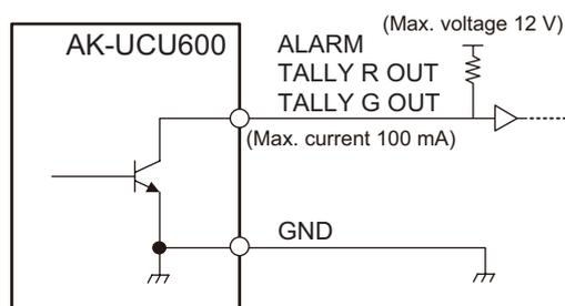
Withstand voltage: 12 V DC max.
