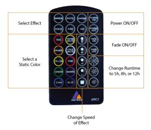
The ARC1 is very handy to switch several lights on or off at a time. The ARC1 can also accept configuration commands that are sent from the AsteraApp $^{TM}$  to a light by pressing the POWER ON button.
