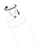
The eyebolts can also be used to suspend the tube but in this case a secondary point must be attached for safety (e.g. via a holder).
