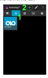
On the AsteraApp™ main screen, first press the Targets button (1) and then the "+" sign (2) to add a new target.
