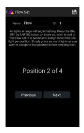
Now your lights will flicker every two seconds. To add a light to the currently shown positon of this set, press its button. Walk through the positions by "Previous" and "Next" and assign your lights. When finished, press the save button on top.
