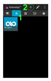
On the AsteraApp™ main screen, first press the Targets button (1) and then the "+" sign (2) to add a new target.
