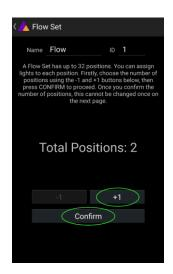
Each flow set can have up to 32 positions. Once the correct number is entered, press "Confirm".
