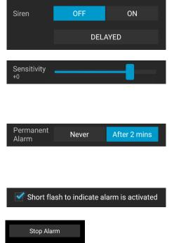
If the siren is set to DELAYED, it sounds only if the alarm persists for more than 6 seconds. The ON setting makes it sound immediately, while the OFF setting mutes it always.
