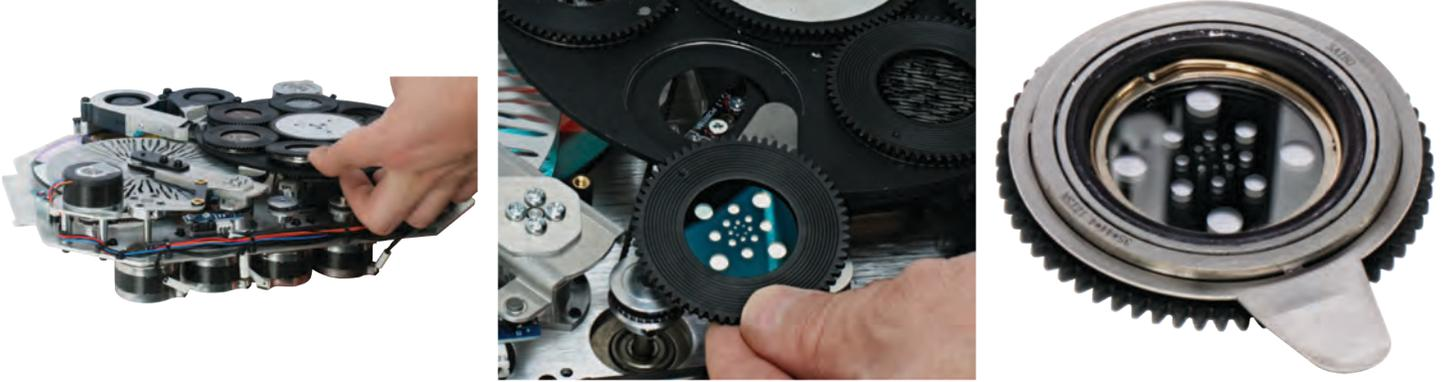
Locate the specific Rotating GOBO to replace. Carefully grip the GOBO using your thumb and index finger, gently lift it slightly, and then pull it out and away until it fully clears the GOBO Wheel.
