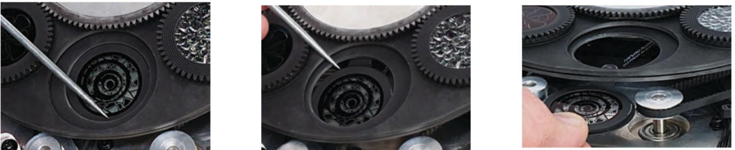
Rotate the Static GOBO Wheel until the desired GOBO is visible through the OPEN slot in the Rotating GOBO Wheel. Using a precision pick (or similar tool), carefully press the Static GOBO Holder down slightly, then using your thumb and index finger, gently pull it out and away until it fully clears the GOBO Wheel.
