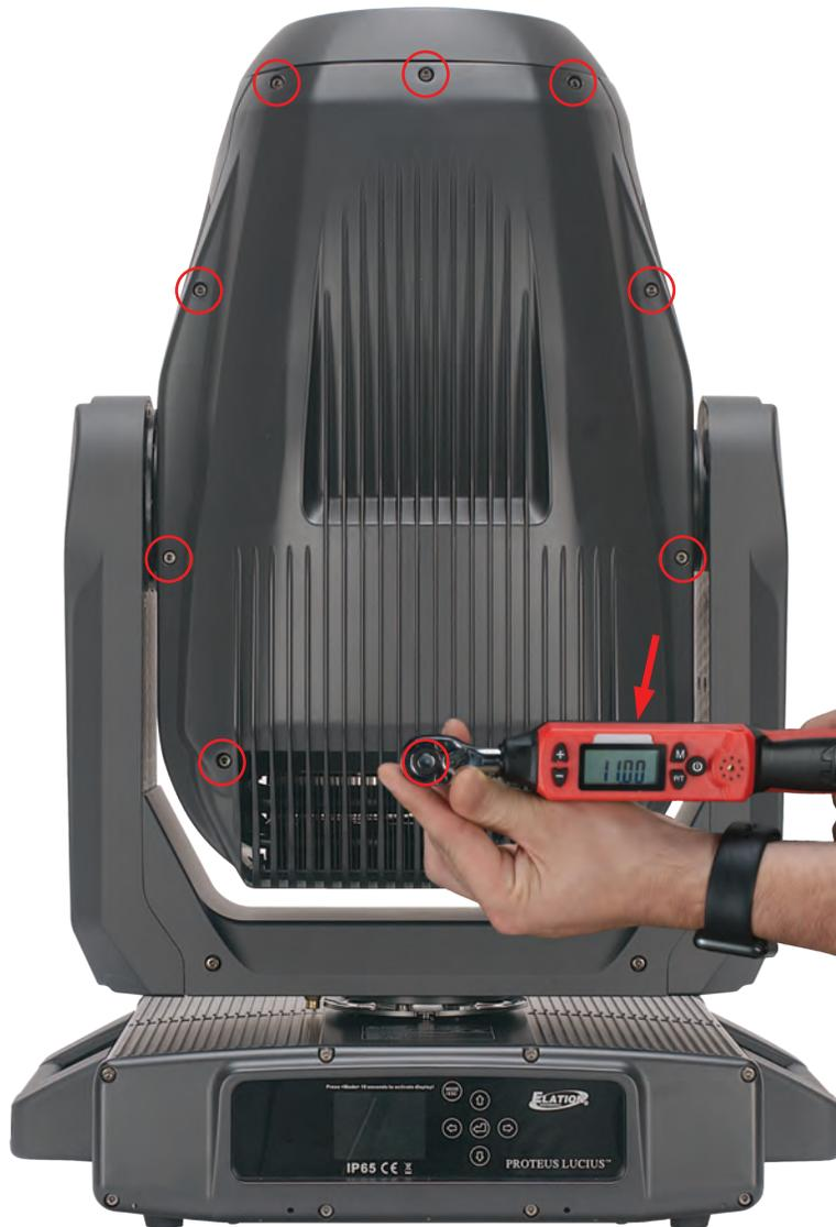
The hex-head screws holding either the panels or the base **MUST** be tightened with a torque wrench (not included). **TORQUE SETTING = 11 lbf-in. (12.7kgf-cm)\***
