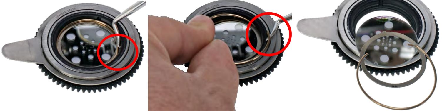
8. Locate the tab of the spring, and with a precision pick (or similar tool), carefully press the retaining spring inward to relieve the tension. Remove the retaining spring and carefully separate the GOBO from the GOBO Holder. Lastly, remove the flat washer attached to the removed GOBO and attach it to the desired replacement GOBO. Install the replacement Rotating GOBO following the steps above in reverse order.
