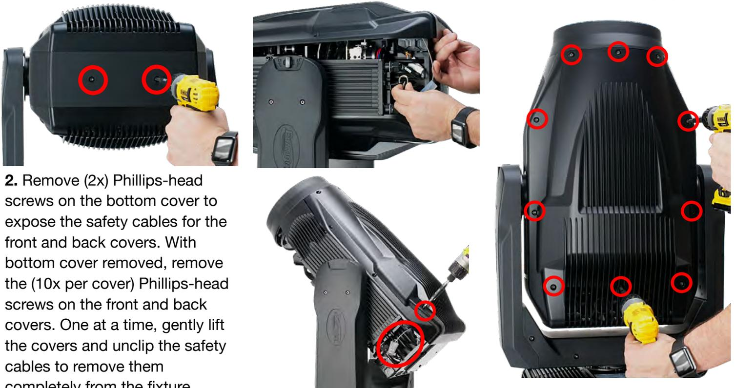
2. Remove (2x) Phillips-head screws on the bottom cover to expose the safety cables for the front and back covers. With bottom cover removed, remove the (10x per cover) Phillips-head screws on the front and back covers. One at a time, gently lift the covers and unclip the safety cables to remove them completely from the fixture.
