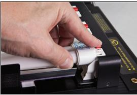
To remove, press red locking tab down and pull up on lamp.
