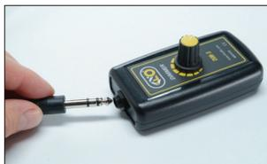
Insert the other end of the dimmer cable into the Diva-Lite Remote Dimmer (**DIM-5**).
