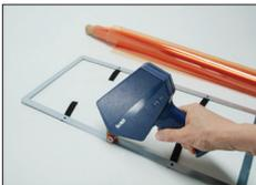
Rotate all Velcro tabs to the inside of frame. Apply double sided transfer tape to one side of the gel frame.
