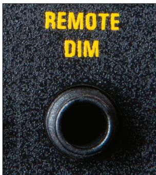
Insert the dimmer cable into the receptacle marked **REMOTE DIM**.
