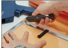
Trim the excess gel from the frame. Rotate Velcro tabs back into position.
