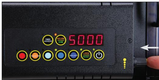
Press the rotating knob once to shift the **Kelvin** profile from **Coarse** to **Fine** increments.
