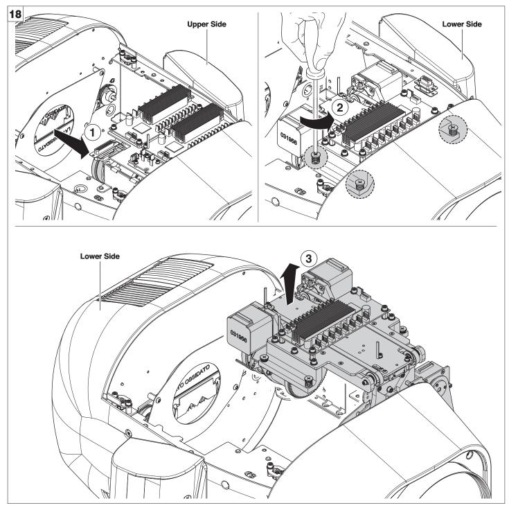
**Extraction of the effect modules -** Fig. 18. **IMPORTANT: Grasp the modules using the support structure and not the details which could get damaged. Insertion of the effect modules:** Repeat the operations indicated in Fig. 14, 15, 16, 17 and 18 in reverse order.
