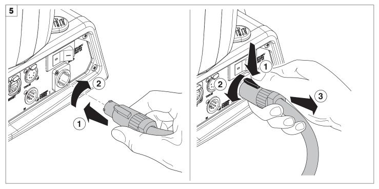
Connecting and disconnecting power cable - Fig. 5
