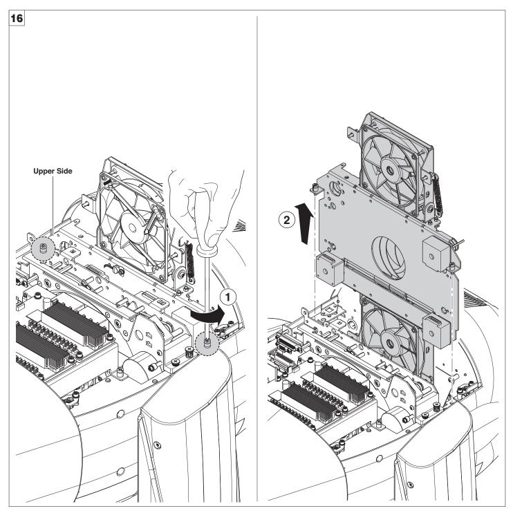
Extraction of the effect modules - Fig. 16. IMPORTANT: Grasp the modules using the support structure and not the details which could get damaged. Insertion of the effect modules: Repeat the operations indicated in Fig. 14, 15, 16, 17 and 18 in reverse order.
