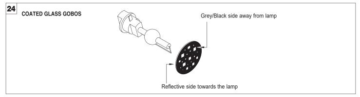
**Gobo orientation** - Fig. 24 The pictures shown the correct gobos orientation.
