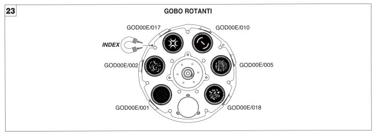
Replacing rotating gobos (ø 32.8 mm - max 23 mm image - thickness 1.1 mm) - Fig. 23
