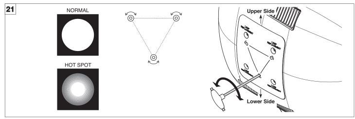
ATT200/001 is the part number of a CP tool, that could help you to take off the lamp from the fixture.
