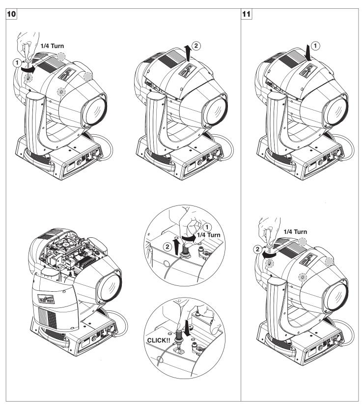
Locking and releasing Pan and Tilt movements - Refer to the instructions in the UNPACKING AND PREPARATION section. Opening the head covers - Fig. 10.
