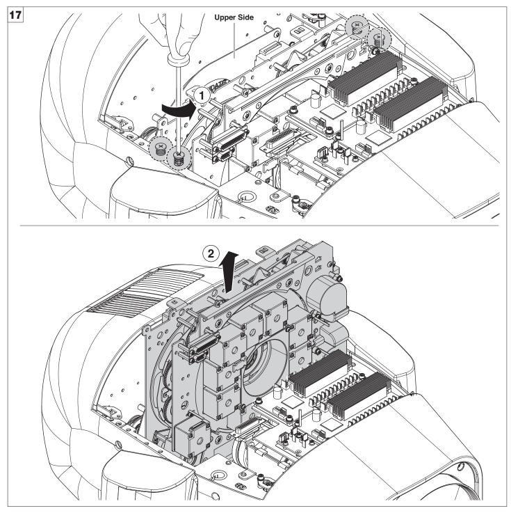
Extraction of the effect modules - Fig. 17. IMPORTANT: Grasp the modules using the support structure and not the details which could get damaged. Insertion of the effect modules: Repeat the operations indicated in Fig. 14, 15, 16, 17 and 18 in reverse order.
