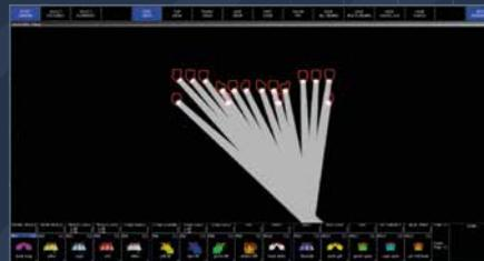
Focus Hold enables focusing of moving fixtures direct from the Plot view onto a single point massively reducing the time taken to create position focus' and enabling easy live tracking of artists' position.
