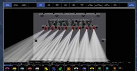
Focus Line enables even more powerful looks to be created by automatically aligning selected fixtures to a flexible line on the plot adjustable in position, orientation and length - this for example enables a group of lights to be fanned across the complete down stage edge at the touch of a button regardless of the physical orientation of the fixtures in the rig.
