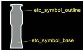
The outline section needs to be tagged as etc\_symbol\_outline0, etc\_symbol\_outline, and/or etc\_symbol\_outline2. The base section needs to be tagged as etc\_symbol\_base0, etc\_symbol\_base, and/or etc\_symbol\_base2. Tags can be layered, and they will render in the order listed below:
