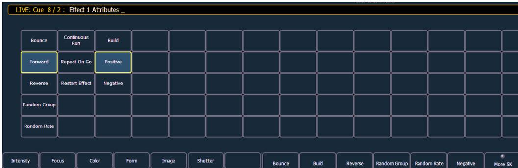
**{Restart Effect}** is an attribute that can only be accessed from this display. When enabled, **{Restart Effect}** will cause an effect to restart whenever the cue is fired. This attribute is applied to the cue that the effect is stored in and not in the effect itself.
