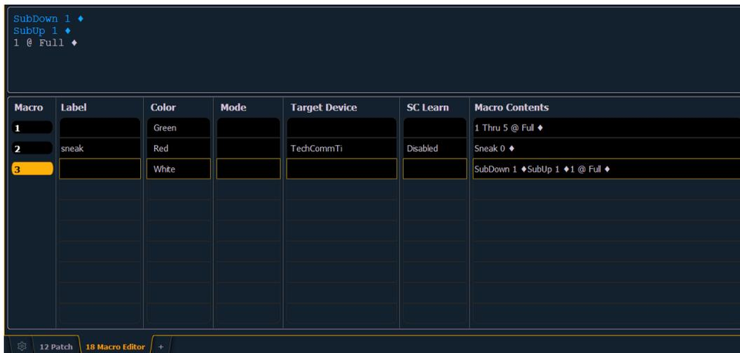
While in the macro editor display, any numeric entry on the command line is assumed to be a macro number. If the macro number entered already exists and **[Enter]** is pressed, the macro list will page to the selected macro and the macro content detail section will display all of the contents of the selected macro. If the macro number entered does not exist in the list and **[Enter]** is pressed, an empty macro will be created with the specified macro number.
