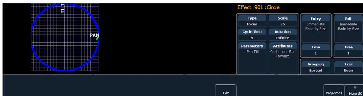
When adjusting the form of a focus effect, you can hold down **[Shift]** while using the horizontal encoder to change the vertical form.
