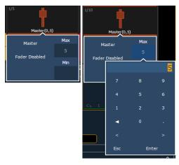
The fader buttons can be assigned as bump, disabled, or macro (see <u>Submaster Fader and Button</u> <u>Configuration (on page 383)</u>). It is recommended that the bottom button be set to bump for turning the fader on/ off. When turned on, the LED will be solid green.
