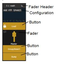
Each fader is color coded based on its assigned target type. Grandmasters and inhibitive submasters are in red, additive submasters are yellow ,playback faders display in green ,and presets, palettes, global effects, and manual time masters are brown.
