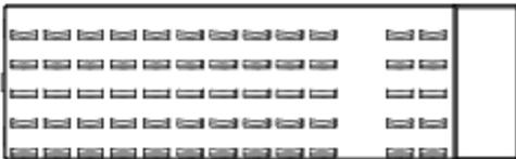
Button modules are available in a 50 button array for use with the direct selects. Button modules provide you with tactile feedback of each button press. The module is transparent allowing the text and graphics from the LCD to repaint each button. Up to three button modules may be installed on the console, two on LCD A and one on the top of LCD B, above the CIA.
