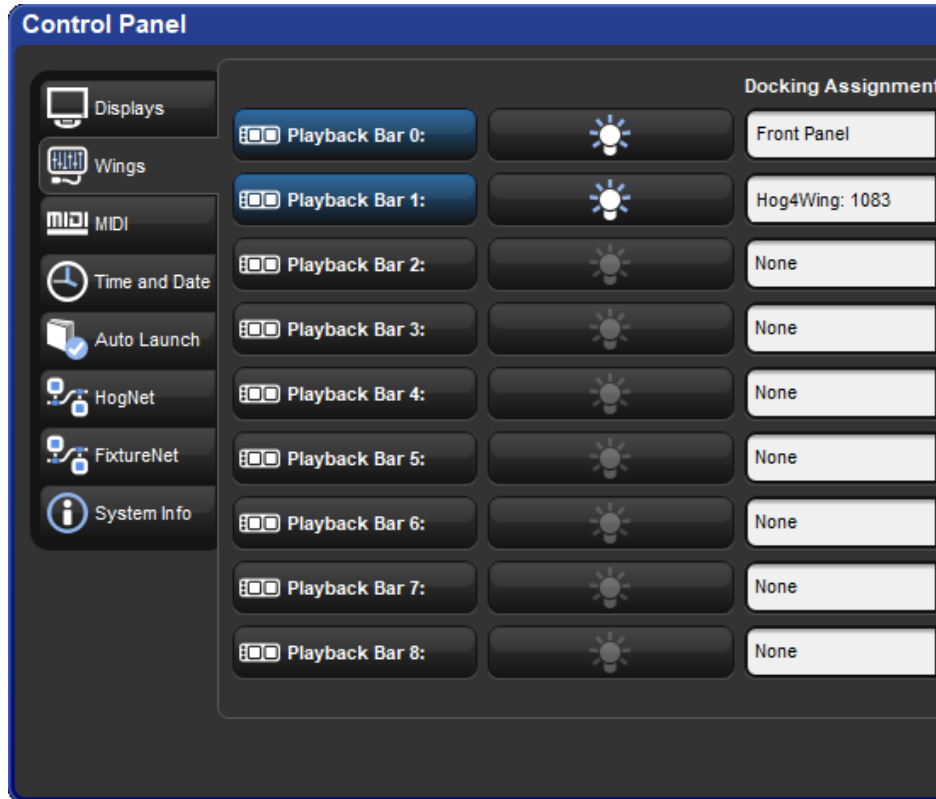
Figure 3.12. Wings pane of the Control Panel with active front panel and wing docking assignments
