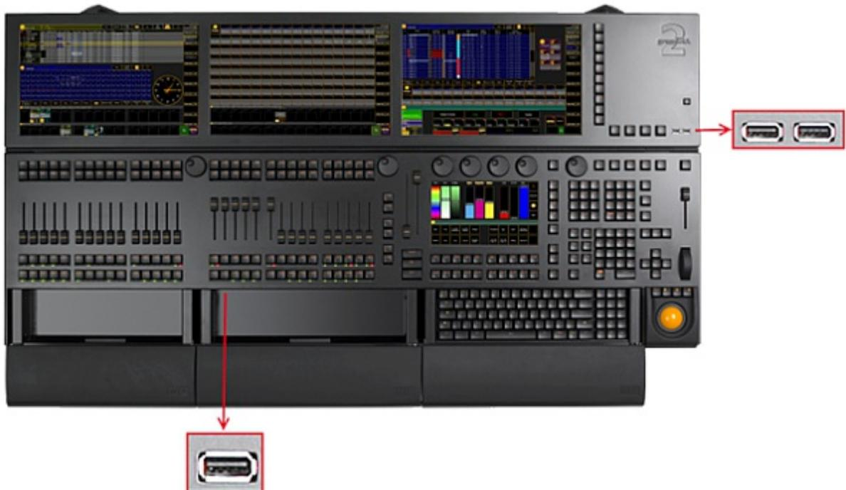
*grandMA2 full-size USB connector front panel*
