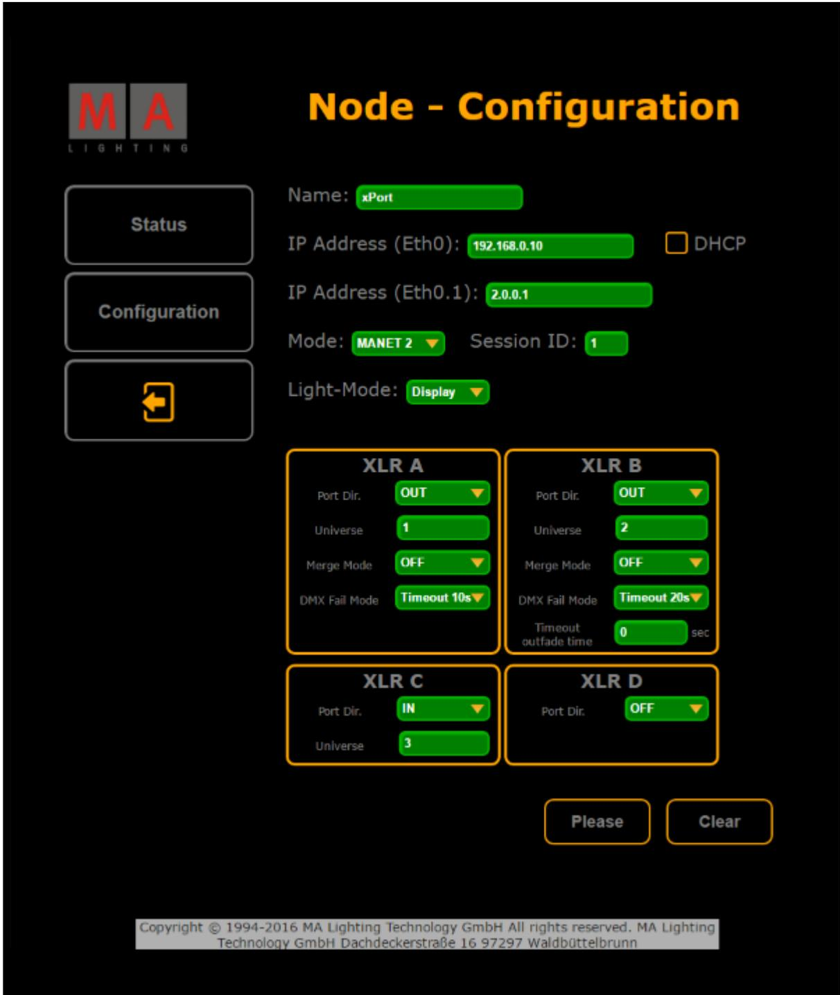
The screenshot shows the 'Node - Configuration' interface for an MA xPort node. On the left, there are three buttons: 'Status', 'Configuration', and a back arrow. The main area contains the following configuration fields:
