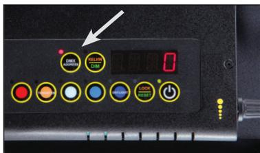
All manual controls are disabled once the DMX cable is applied and DMX is turned on.
