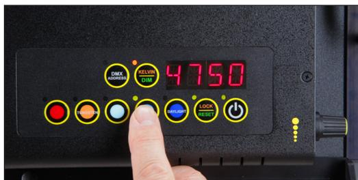
The setting can be assigned to any preset button by holding down the desired button for 5 seconds.
