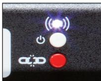
Press the white Power/Wireless button. A blue light indicates fixture is ready to link to transmitter.
