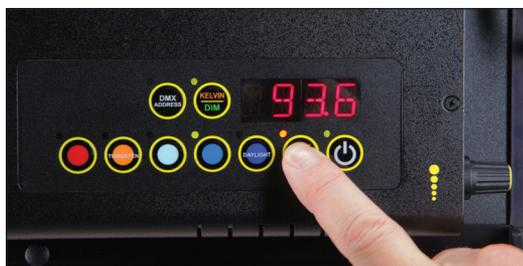
Press the **LOCK / RESET** button to lock the Kelvin and Dim settings. An amber indicator will display in **LOCK** mode.
