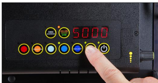
To reset factory settings, press and hold the **LOCK / RESET** button for 5 seconds.
