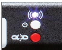
To unlink from the fixture: Press and hold the red unlink button for 3 seconds. A blue light is displayed when unlinked.
