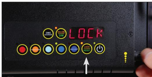
In **LOCK** mode, controls are disabled and **LOCK** will appear in the display.
