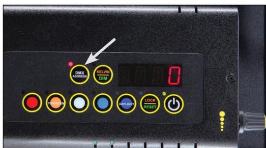
Press and hold the **DMX ADDRESS** button to select a DMX address. The displayed number will flash while in edit mode.
