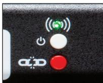
Press the link/unlink button on the transmitter to link to the Celeb 401Q. A fast red blinking light is displayed while searching for signal. A slow green blinking light\* displays when linked.
