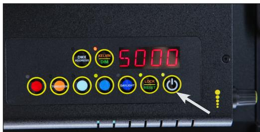
Press the **On/Off** button to turn on the fixture. The display will show its last setting.
