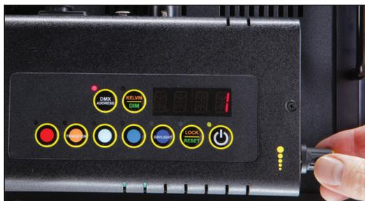
Turn the dimming knob to select a valid address from 1-512. (Note: 0 or 513-999 are invalid addresses.)
