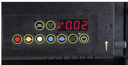
When power is first applied to the fixture, the alphanumeric display shows the current software version.
