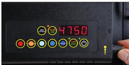
In **KELVIN** mode, the Kelvin can be fine tuned with the adjustment knob to custom settings between 2700K to 6500K.
