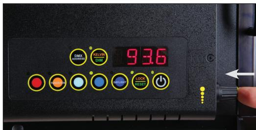
Press the rotating knob once to shift the **Dim** profile from **Coarse** to **Fine** increments.
