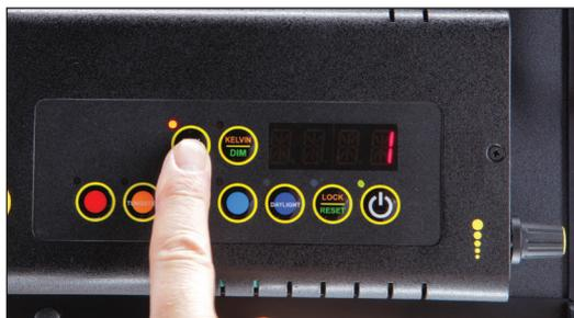
To save the DMX channel, press the **DMX ADDRESS** button again. When set, the displayed number will stop flashing.
