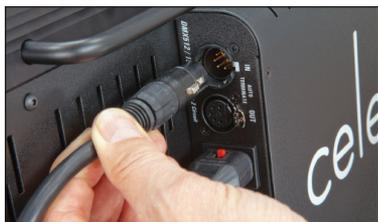
**Note:** When operating fixtures at great distances from the dimmer board, it is recommended to use Opto-Isolators to provide DMX signal amplification.
