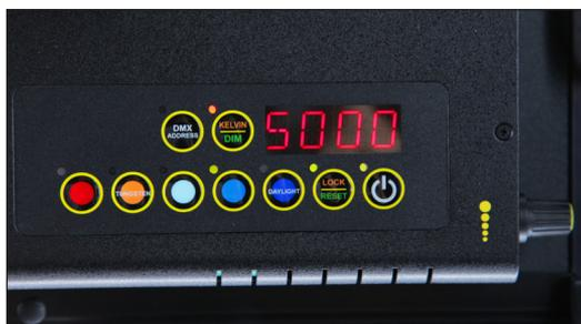
The Celeb 401Q DMX operates on two DMX channels using DMX512. The first channel operates dimming; the 2nd channel operates Kelvin color temperature control.
