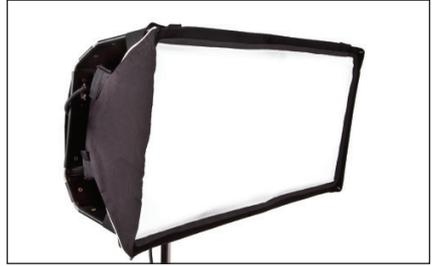
The SnapBag accessory (**DFS-FS31-S** & **DFS-FS21-S**) is a lightweight fabric tailor-made for the Select LED. It slips over the fixture and is attached with straps. The reflective material intensifies the soft light. The removable Magic cloth or Grid cloth attaches to the inside with Velcro.
