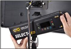
Insert the 4 rubber feet of the controller into the 4 holes in the fixture.
