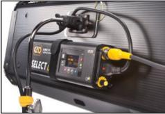
Connect the harness to the Controller. Align the key ways on the harness connector with the circular receptacle on the ballast. Rotate the silver locking ring until it clicks into the lock position.
