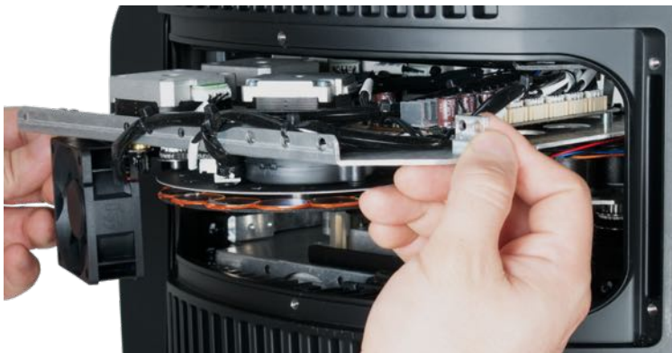
9. Carefully remove the effect module from fixture.
