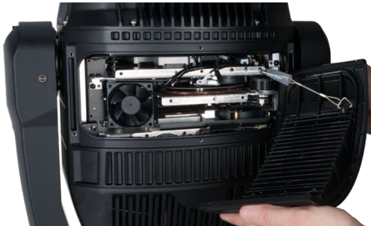
5. Unclip the panel safety cable on the opposite side of the head.
