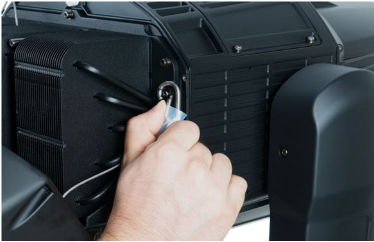
4. Unclip the rear cover safety cable.
