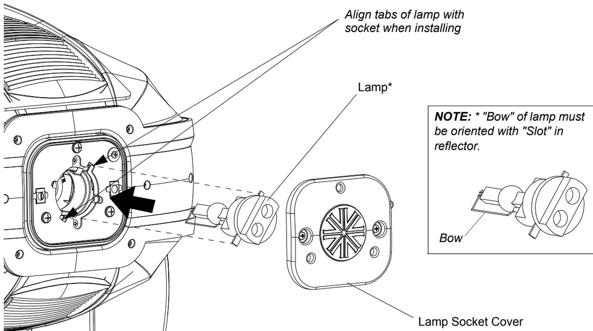
**Figure A-2: Lamp Installation**
