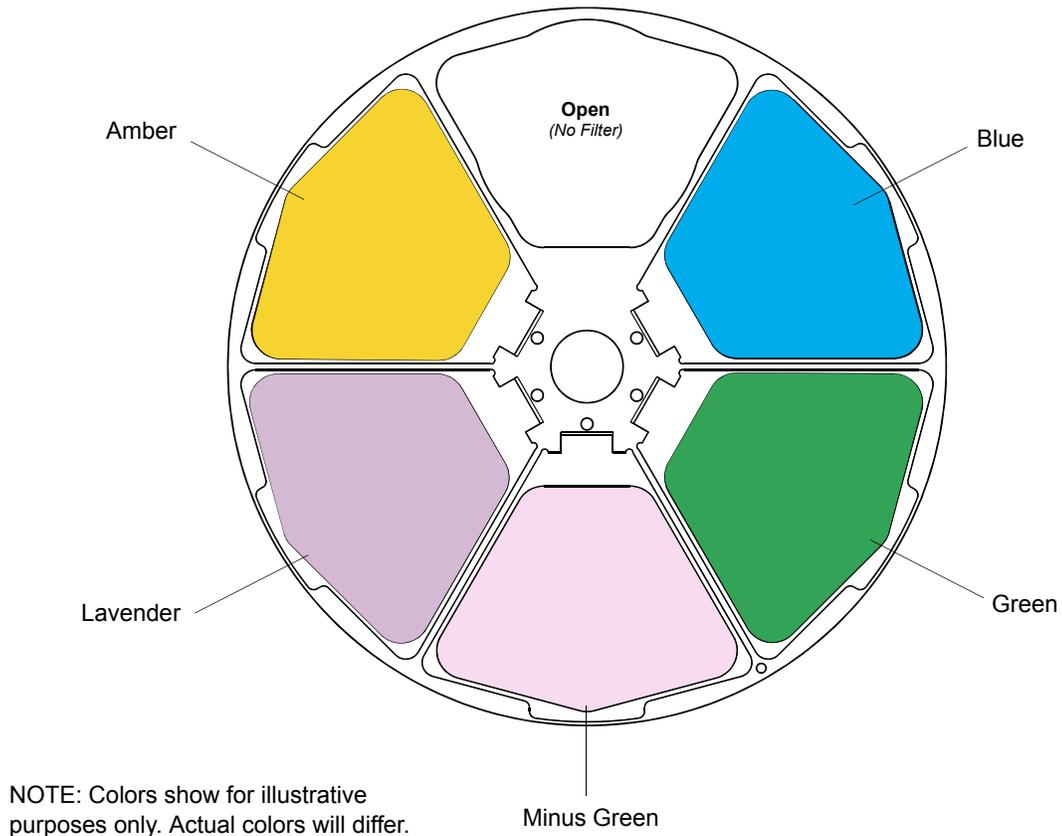
Figure 3-2: VL4000 BeamWash Fixed Color Wheel 2
