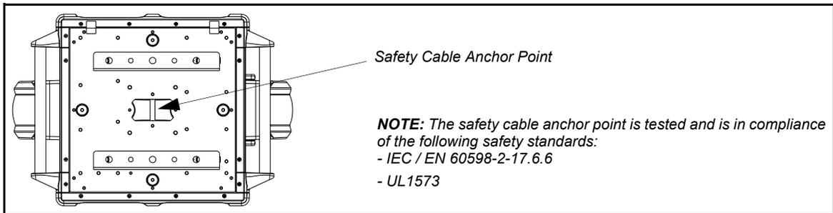
**Figure 2-9: Safety Cable Installation / Luminaire Hanging**
