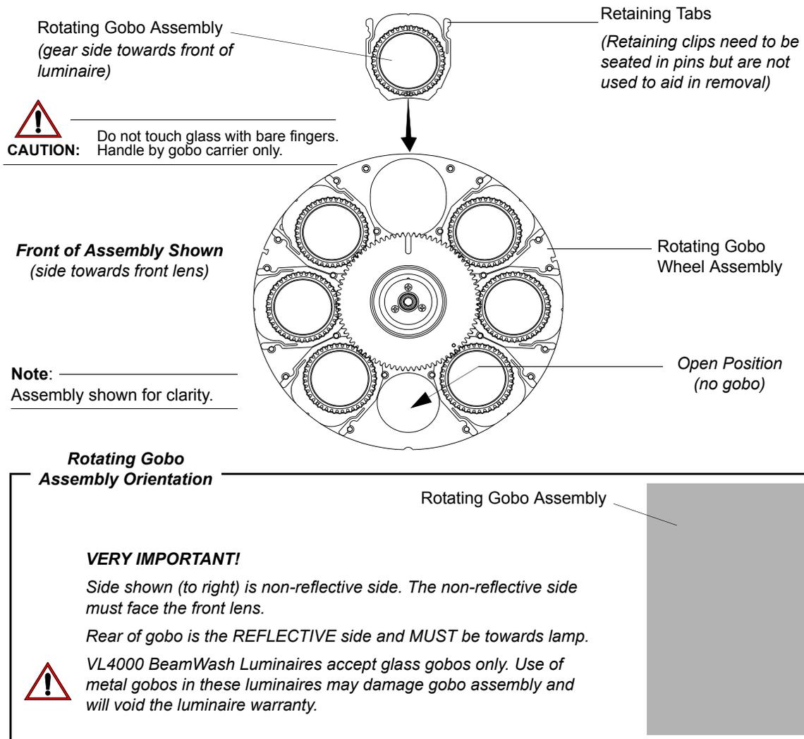
**Figure A-9: Rotating Gobo Wheel - Gobo Installation**
