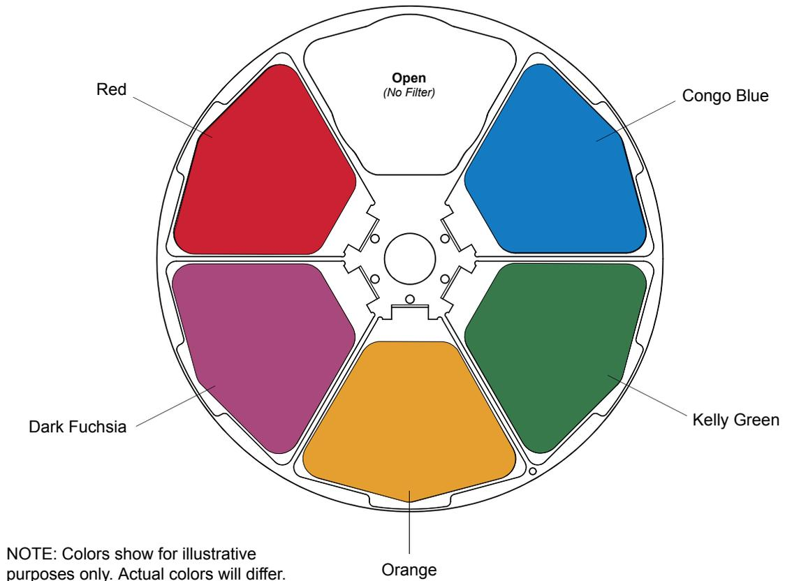
Figure 3-1: VL4000 BeamWash Fixed Color Wheel 1
