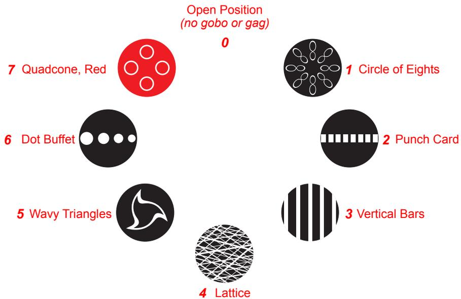
**Figure 3-4: Rotating Gobo Wheel 2 - Standard Gobo Load**
