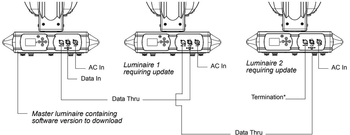
\*DMX terminator required for last fixture on DMX line.
