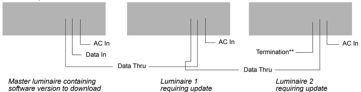
\*\*DMX terminator required for last fixture on DMX line.
