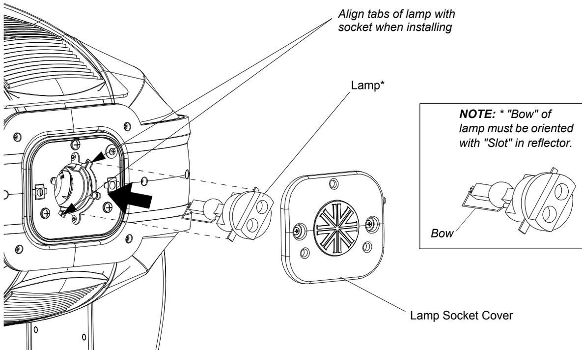
**Figure 2-3: Lamp Installation**
