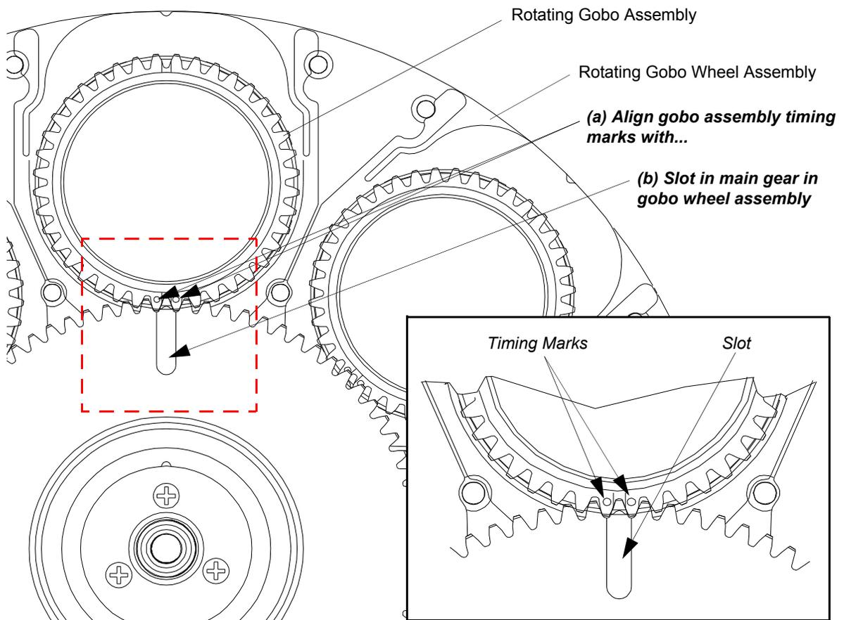
Figure A-8: Rotating Gobo Wheel - Gobo Clocking
