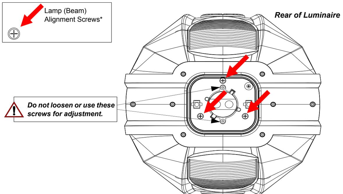
NOTE: \*Lamp Socket Cover removed for clarity. It is not necessary to remove Lamp Socket Cover to align lamp.
