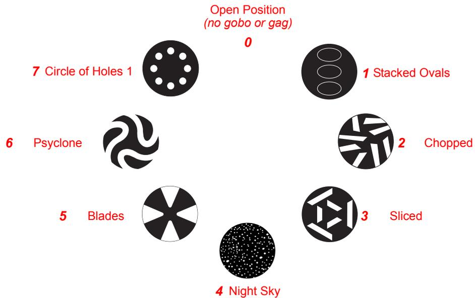
**Figure 3-3: Rotating Gobo Wheel 1 - Standard Gobo Load**
