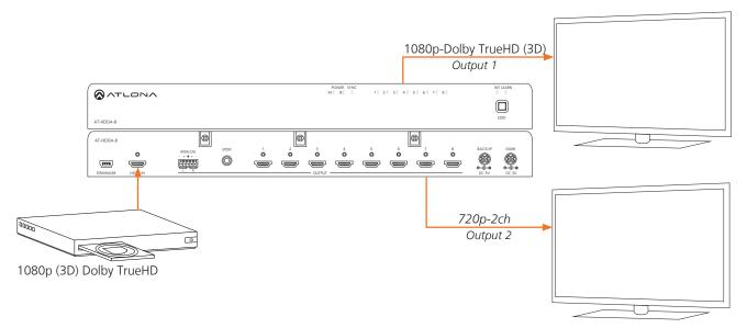
EDID learn mode loads the highest supported resolution and audio format between output 1 and the source then mirrors it to all outputs. \*EDID learning is only available for output 1\*
