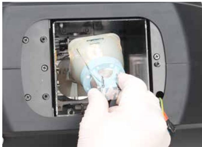
7. Using two fingers, gently install new lamp into the fixture. (See above)
