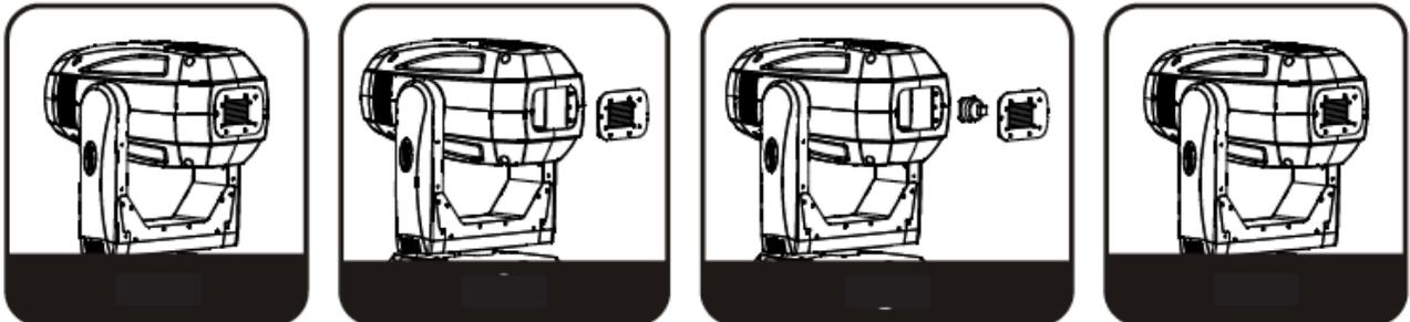
1. Place fixture on a flat surface and remove (3) screws marked "A", "B", and "C" and then remove lamp cover to access the lamp. (See below)
