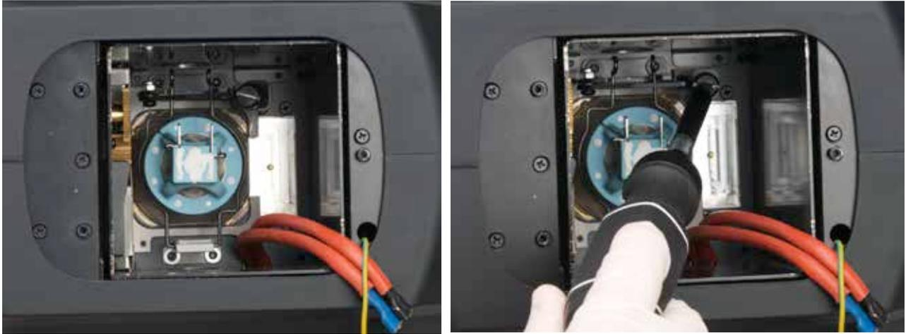
10. Gently attach **(2) Wires** to spade terminals on the base of the lamp. (See below)
