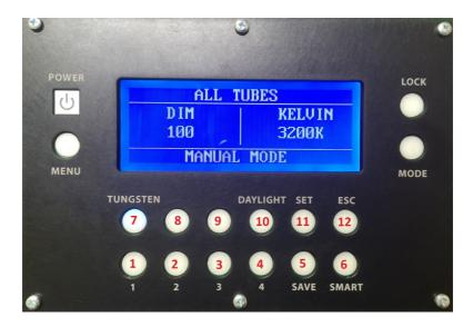
POWER: Turns the LCD Controller on & off.
