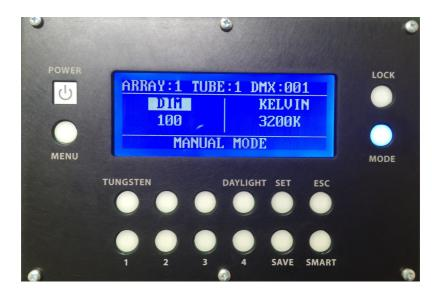
Each **ARRAY** consist of a set of four tubes. You have the ability to control each individual tube within each **ARRAY** (see page 4). Depending on your fixture model you could have anywhere from 1-5 **ARRAYS**.
