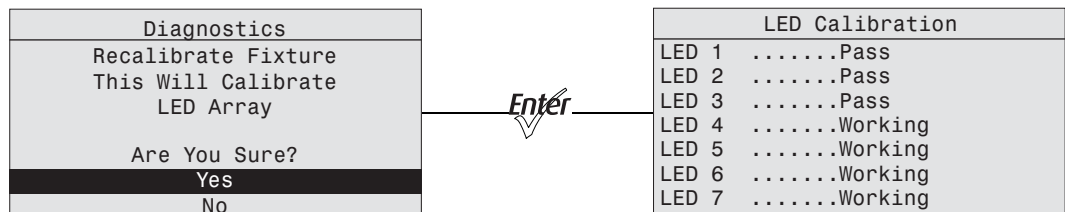
Figure-3.36 LED Calibration Screen with Calibration in Process.
