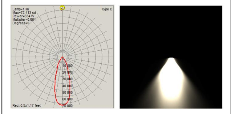
IMPORTANT POINTS: LUMINAIRE OUTPUT: 32211 LM POWER : 834W Measurement in Cd: 72413 cd
