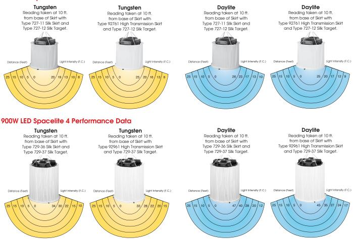
\* Light tapers smoothly at edge of field. Dimensions listed define flat area boundaries at which the intensities are approximately 50% of tabulated intensities at beam center.
