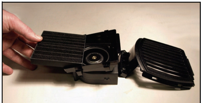
Figure 15: Head air filter alignment
