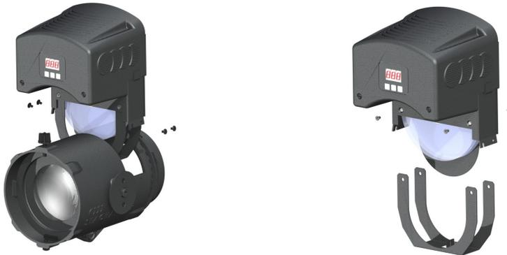
The filters can be easily accessed by removing (4) Philips screws and pulling the protective cage away from the color engine as shown below:
